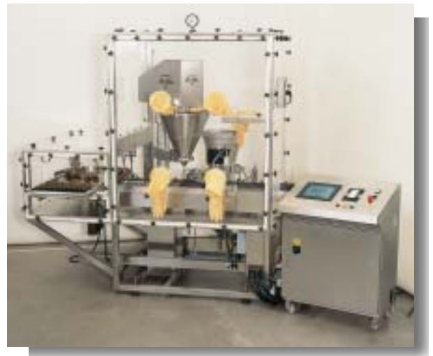
Integrated unscrambling filling and stoppering system in fully sealed glovebox enclosure for precise gravimetric filling of biological analysis samples into vials and small bottles.
