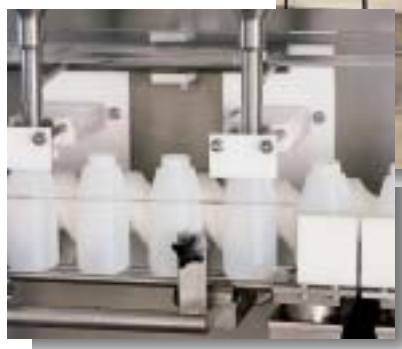
4 head filler for oral suspension antibiotics, the 1 st twin head filling the carrier, the 2 nd twin filling the active. Features: servo worm-scroll bottle transport, neck-entry filling, 100% weight validation/reject, vacuum conveyor hopper feeds, balcony design, touch-screen control.
