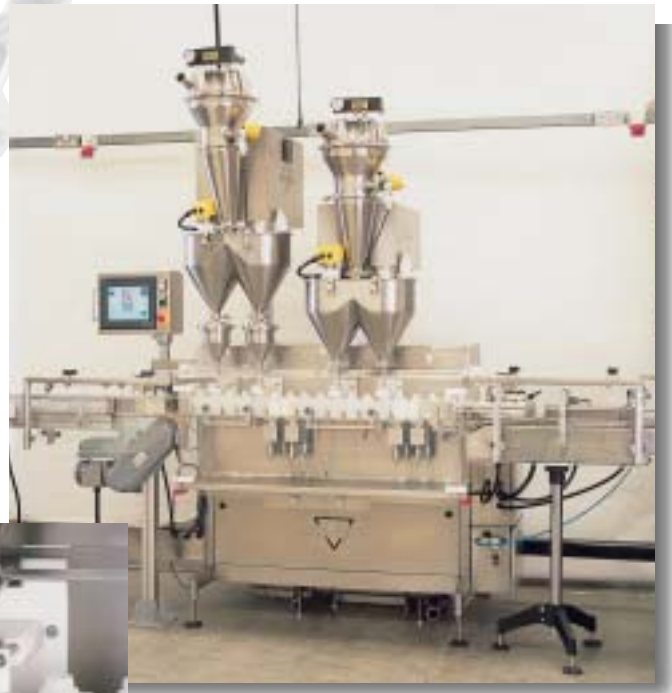
4 head filler for oral suspension antibiotics, the 1 st twin head filling the carrier, the 2 nd twin filling the active. Features: servo worm-scroll bottle transport, neck-entry filling, 100% weight validation/reject, vacuum conveyor hopper feeds, balcony design, touch-screen control.
