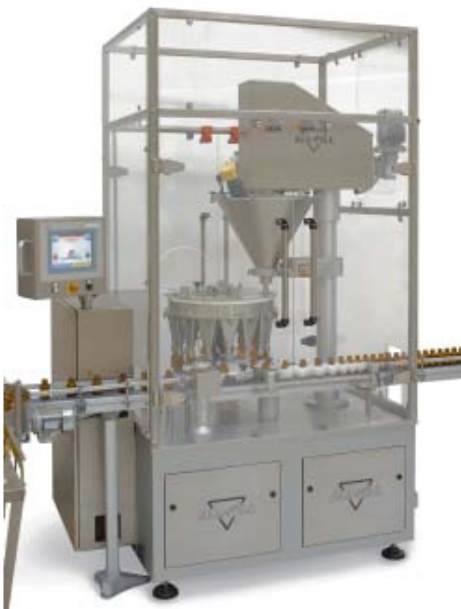
12 Pocket Continuous Motion Rotary with continuous dosing, filling, 6g to 30g dry suspension antibiotics into glass bottles at 8000 bottles per hour.
